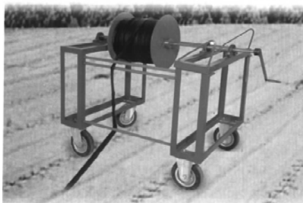
Figure 2. Drip-tape collector device.
