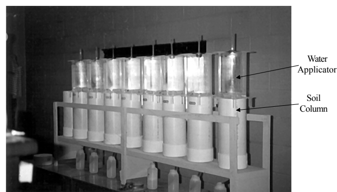
Figure 1. Experimental setup of soil columns and rainfall simulators.
